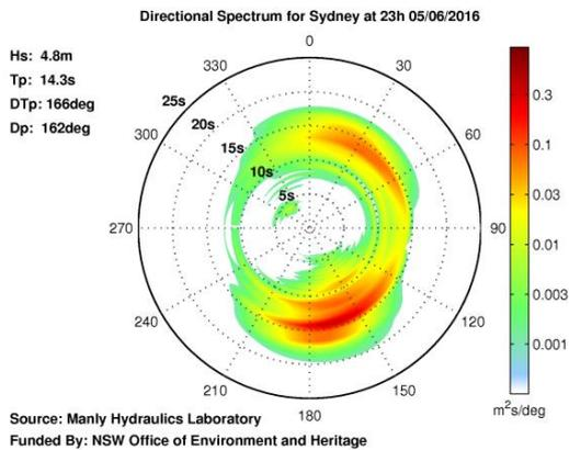
**Figure 4 (a) Directional spectra indicating bi modal nature of storm recorded at the Sydney buoy on 5 June 2018**
