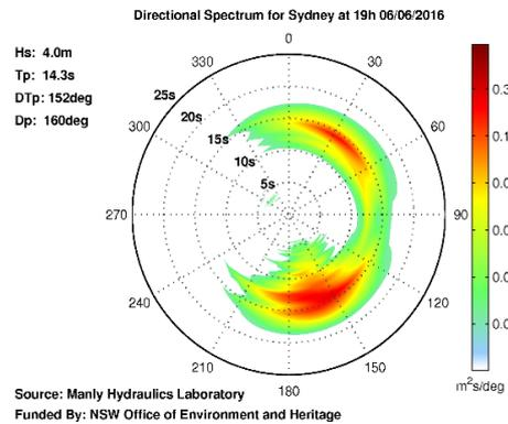
**Figure 4b Directional spectra indicating bi-modal nature of storm recorded at the Sydney buoy on 6 June 2018**
